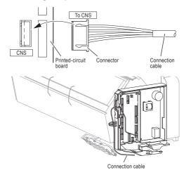
Connect the indoor unit connection cable to the indoor control printedcircuit board.
