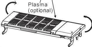
Open the panel and take down the Plasma filter by holding the upper of the Plasma and lifting it upwards according to the arrows.
