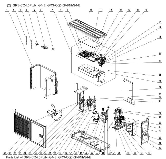
No. Name Quantity Condenser Assy Temperature Sensor Temperature Sensor Strainer Display Board Receiver Board Electric Box Assy Main Board Radiator Top cover Leaded PFC Inductance Main Board mounting card(main board) Main Board Bipolar AC Contactor Terminal Board Terminal Board
