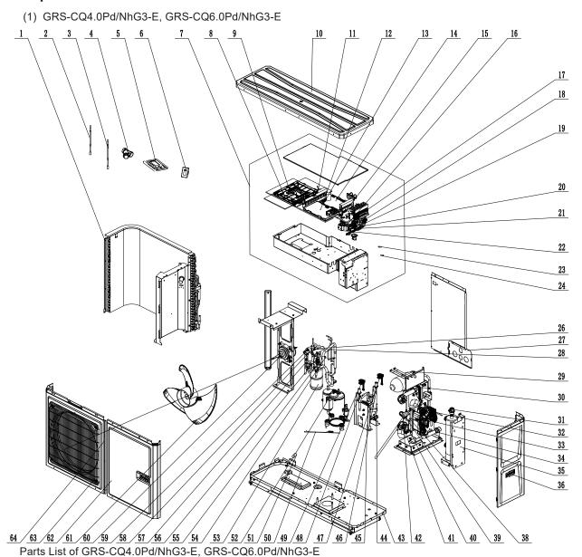
Name Quantity Condenser Assy Temperature Sensor Temperature Sensor Strainer Display Board Receiver Board Electric Box Assy Main Board Radiator Top cover Leaded PFC Inductance Main Board mounting card(main board) Main Board Bipolar AC Contactor
