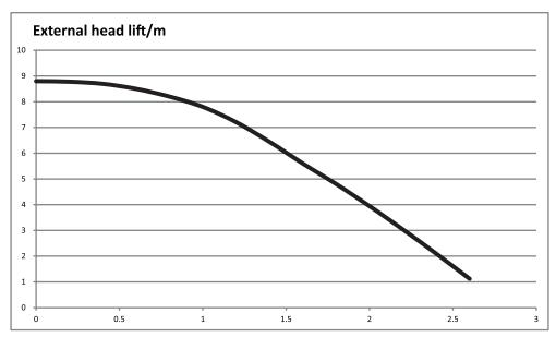
**Notes**(a) See the curve above for the maximum external static pressure. The water pump is of variable frequency. And during operation, the water pump will adjust its output based on the actual load.
