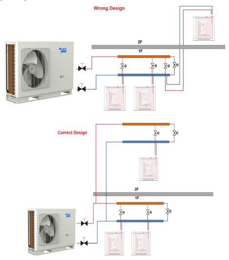
(5) Distance between the unit and the water manifold should be within 15m. If the distance exceeds 20m, then it is required to calculate the hydraulic power.
